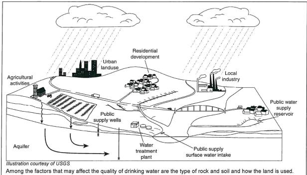
Among the factors that may affect the quality of drinking water are the type of rock and soil and how the land is used. While some rain and snow evaporates into the sky, most of it runs off into nearby rivers and streams or seeps into the ground. Drinking water comes from underground aquifers or surface water bodies.
